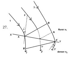
Let XY be interface of two mediums and c<sub>1</sub> and c<sub>2</sub> are velocity of light is rarer and denser medium respectively.
